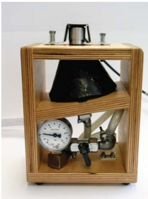
Fig. 7a. Real Beatti – Block test stand for acoustic emission transducer
